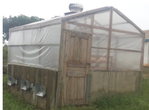
Figure 2. Solar Ten dryer
